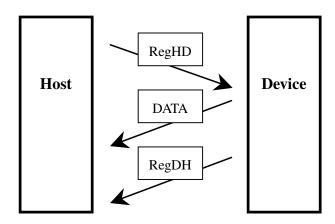
Figure 5.16 DMA data-in command protocol
